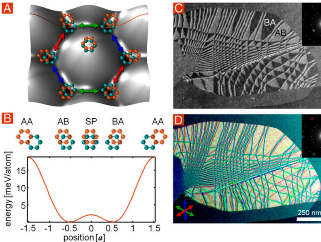
Strain solitons and topological defects in bilayer graphene. PNAS, 2013, Alden, . . . , McEuen
