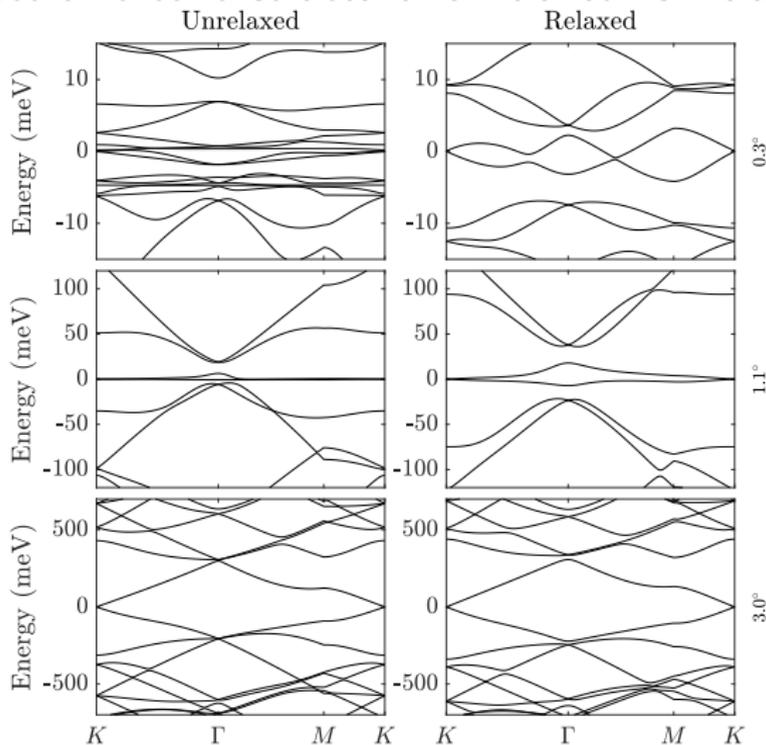
**Figure:** Electronic band structure along high-symmetry lines of the moiré Brillouin zone at a single monolayer  $K$  valley for  $0.3^\circ$  (top),  $1.1^\circ$  (middle), and  $3.0^\circ$  (bottom).
