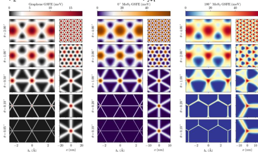
**Figure:** Relaxation results for twisted bilayers with five incommensurate twist angles each. The left panel of each column shows  $F_{\text{GSFE}}(\mathbf{b} + 2\mathbf{u}(\mathbf{b}))$  over  $\Gamma$  (the relaxation pattern in configuration space) and the right panel shows  $F_{\text{GSFE}}(\mathbf{r})$  (over real space).
