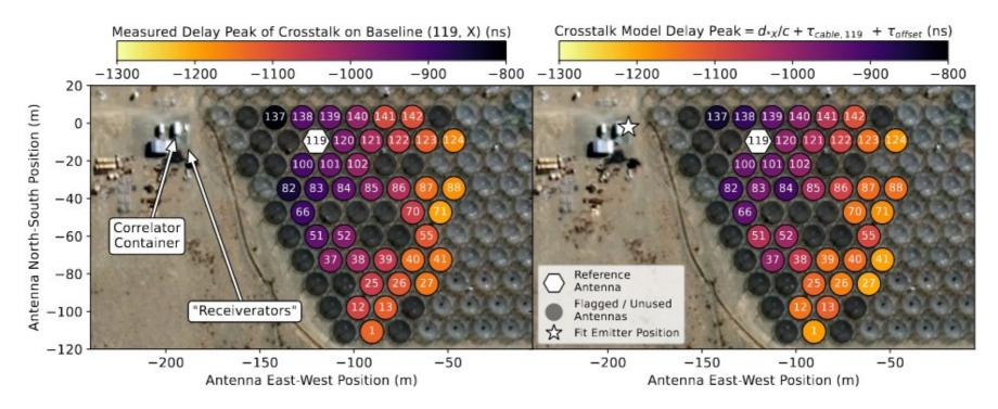
Antenna  $\rightarrow$  150m cable  $\rightarrow$  amplifiers in receiverator  $\rightarrow$  broadcast back to antennas
