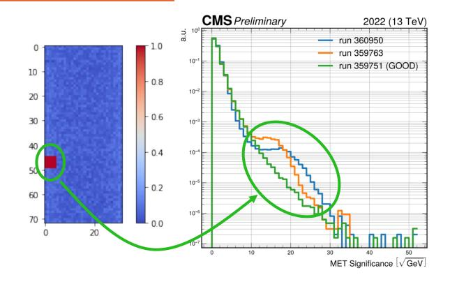
As an example: a noise-dominated channel in the hadronic calorimeter leads to anomalies in the distribution of missing transverse energy (MET) related quantities
