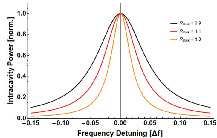
The cavity mode we want to lock on gets sharper with laser gain (i.e. laser power)!
